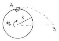
(a, 4 points) What is the initial velocity  $\mathbf{v}_0$  of the chip at point A when it separates from the disc?
