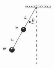
(b, 16) Either section of the rod will break if subjected to a tension force of 4.2mg or greater. In the motion described above, does either section break? If so, find the angle at which it breaks.
